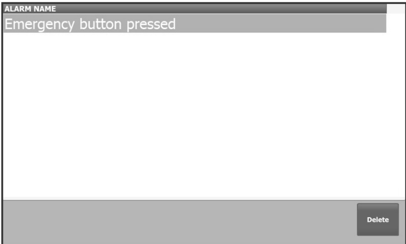
Appearance of the snow cannon operator panel - failure screen
